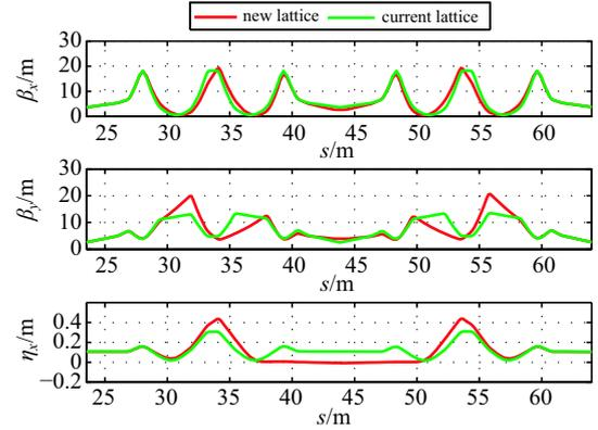
Fig. 4. (color online) Optics of the two cells adjacent to the SW.
