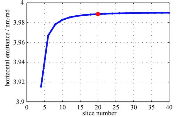
Fig. 2. (color online) Horizontal emittance as an object of slice number per magnetic field period.
