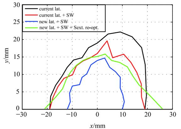
Fig. 5. (color online) Dynamic aperture of different schemes with 1000 turns tracking with AT.
