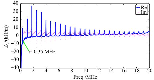
Fig. 13. (color online) Vertical impedance of the kicker with the cable open.
