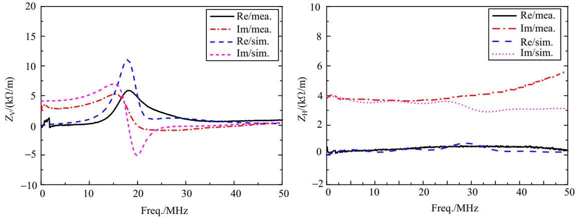
Fig. 14. (color online) Simulated and measured transverse impedance of kicker magnet.
