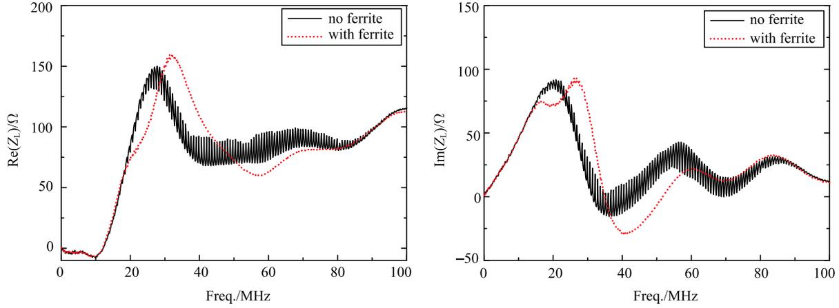
Fig. 6. (color online) Longitudinal impedance of the kicker with and without the ferrite ring.
