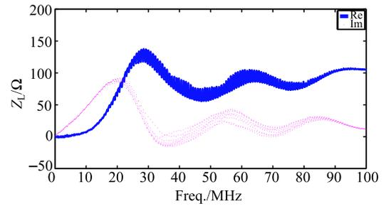
Fig. 5. (color online) Longitudinal coupling impedance of the kicker system.
