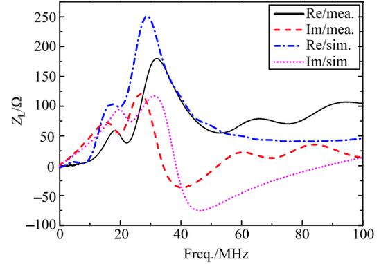
Fig. 4. (color online) Longitudinal coupling impedance of the kicker magnet.
