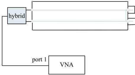
Fig. 9. Schematic setup of the transverse impedance measurement with the loop.
