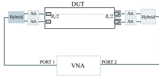
Fig. 7. Schematic view of transverse impedance measurement by the twin-wire.
