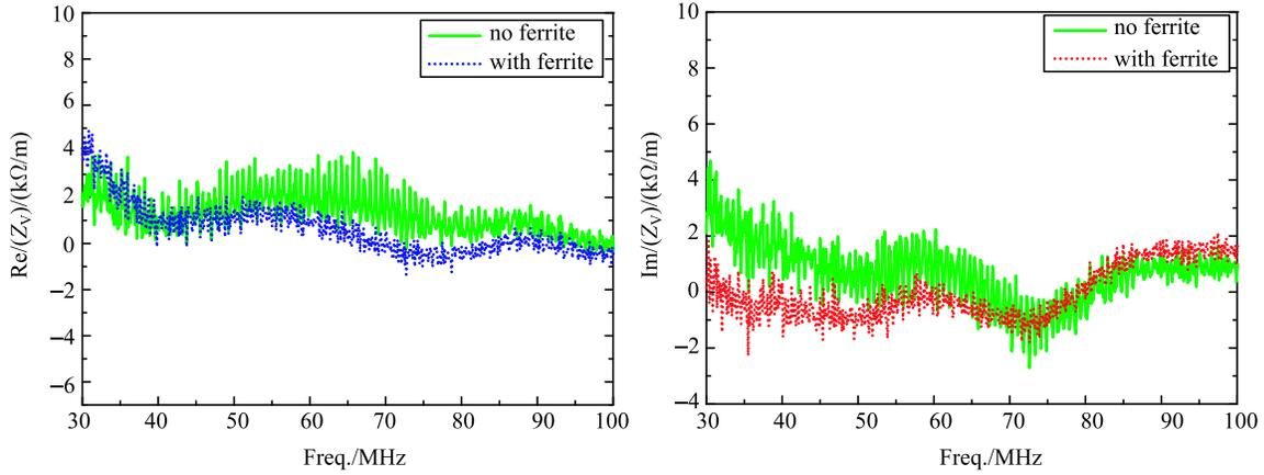
Fig. 15. (color online) Vertical impedance of the kicker system with and without the ferrite ring.
