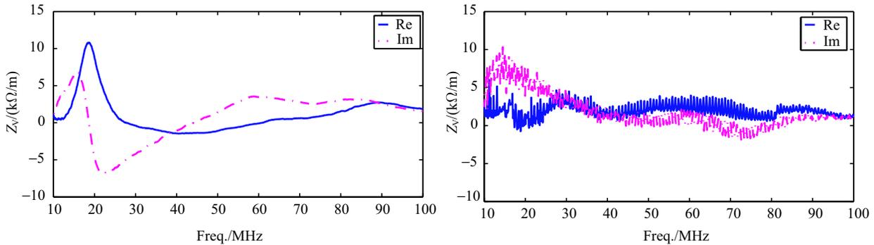
Fig. 8. (color online) Vertical impedance of the kicker magnet (left) and the kicker system (right).
