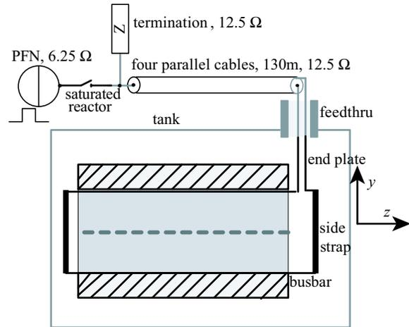
Fig. 1. Schematic view of the CSNS/RCS kicker system.
