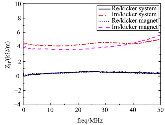
Fig. 10. (color online) Measured horizontal impedance of the kicker by loop.
