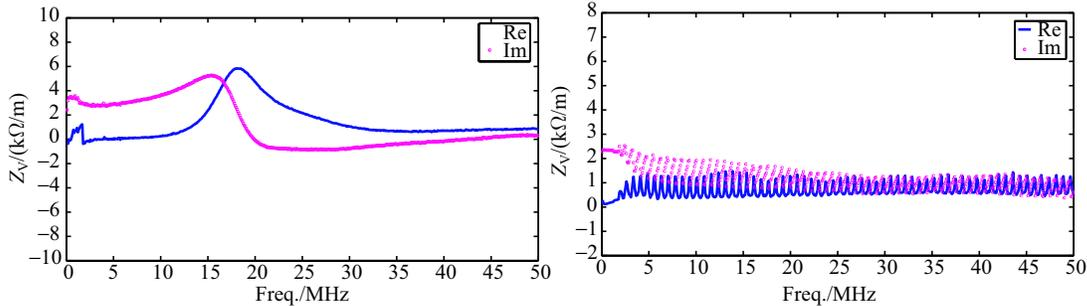
Fig. 11. (color online) Measured vertical impedance of the kicker magnet (left) and the kicker system (right) by loop.
