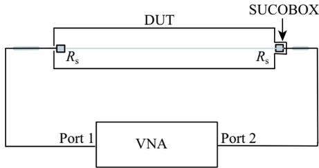
Fig. 3. Schematic setup of the longitudinal coupling impedance measurement.
