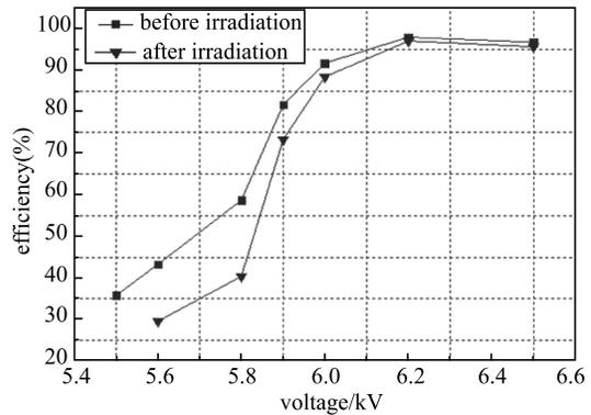
Fig. 4. Efficiency as a function of high voltage before and after irradiation.
