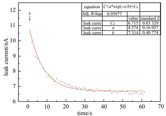
Fig. 12. (color online) Current recovery curve after 36 days of irradiation.
