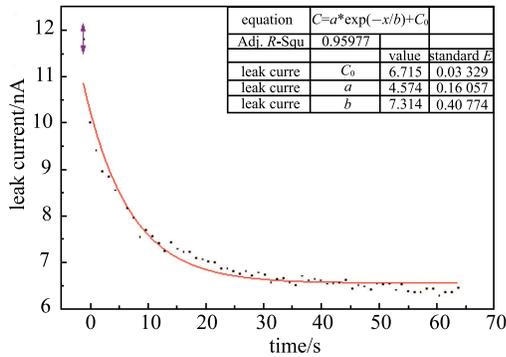
Fig. 11. (color online) Current recovery curve after one day of irradiation.
