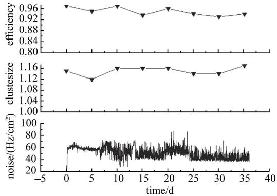
Fig. 8. Variation of efficiency, cluster size and noise with irradiation time.
