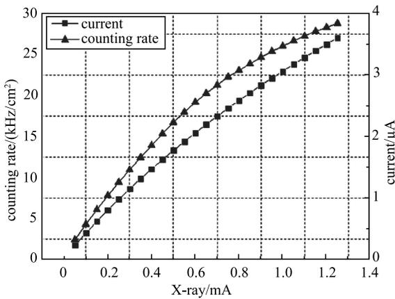
Fig. 6. Variation of current and counting rate with X-ray strength.
