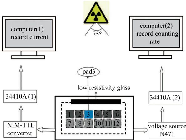
Fig. 2. (color online) Schematic diagram of the monitoring system.
