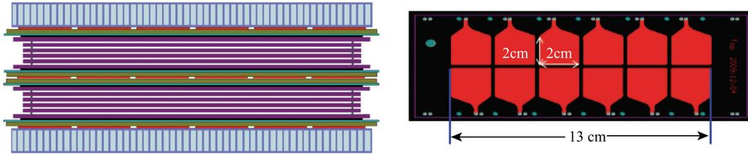
Fig. 1. (color online) Structure of high rate MRPC module.
