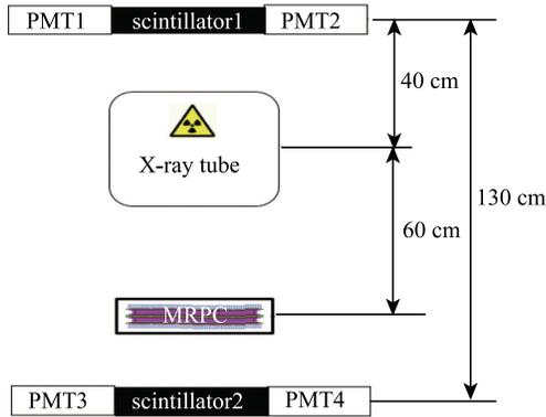
Fig. 3. (color online) Layout of the irradiation system.
