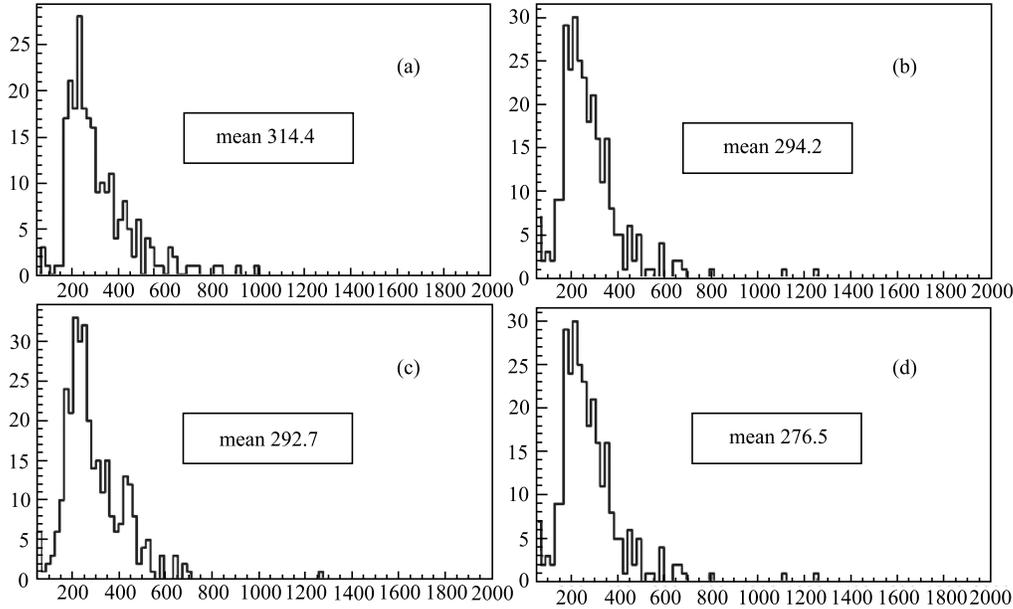
Fig. 10. The charge spectrum at different stages: (a) before irradiation, (b) after ten days' irradiation, (c) after twenty days' irradiation and (d) after thirty days' irradiation.
