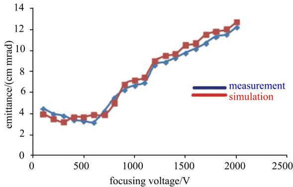
Fig. 13. (color online) Measured and simulated emittance as a function of focusing electrode voltage.
