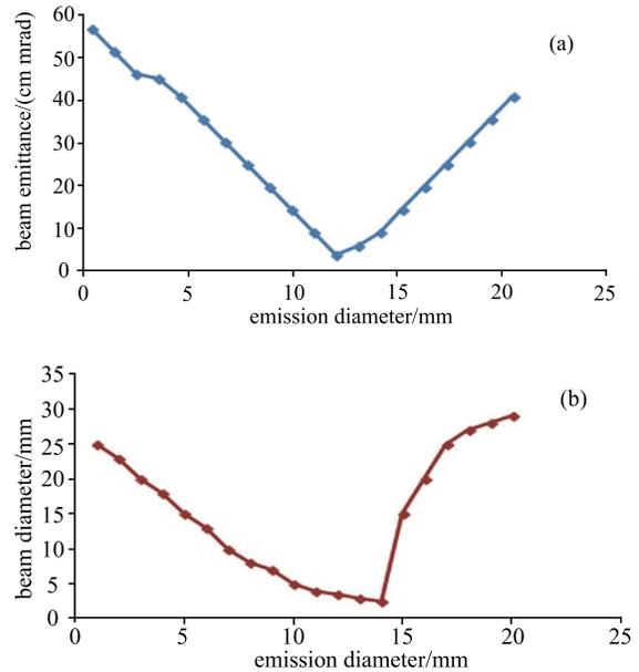
Fig. 8. Beam emittance (a) and beam diameter (b) as a function of the emission electrode diameter for the electron gun system.
