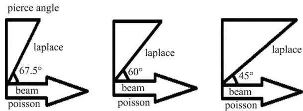
Fig. 5. Different inclination angles of emission electrode.
