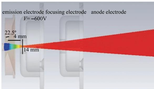
Fig. 9. (color online) Simulation run for the electron gun accelerator structure.
