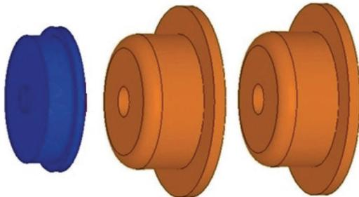
Fig. 3. (color online) Schematic of thermionic electron gun.
