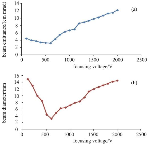
Fig. 6. Influence of the voltage applied to the focusing electrode on both beam emittance (a) and beam diameter (b) of the electron gun.
