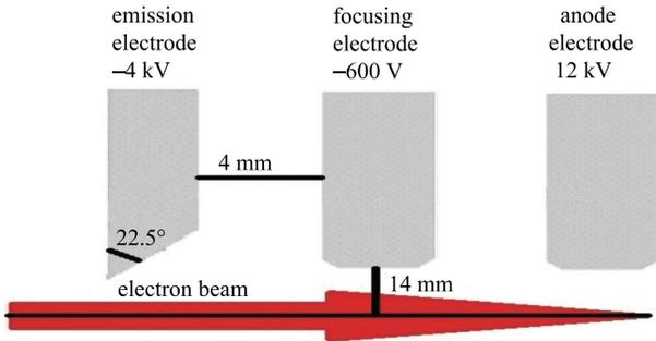
Fig. 2. (color online) Electron gun geometry elements assumed for the CST calculations.
