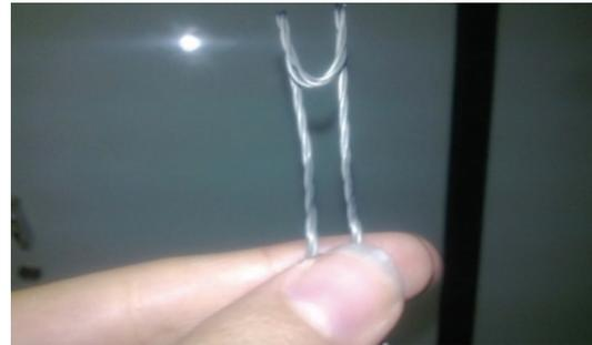
Fig. 1. (color online) Tungsten filament of electron gun.
