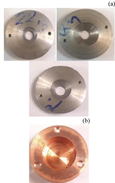
Fig. 10. (color online) (a) the emission electrodes for the three angles ( $22.5^\circ$ ,  $30^\circ$  and  $45^\circ$ ) and (b) focusing and anode electrode.
