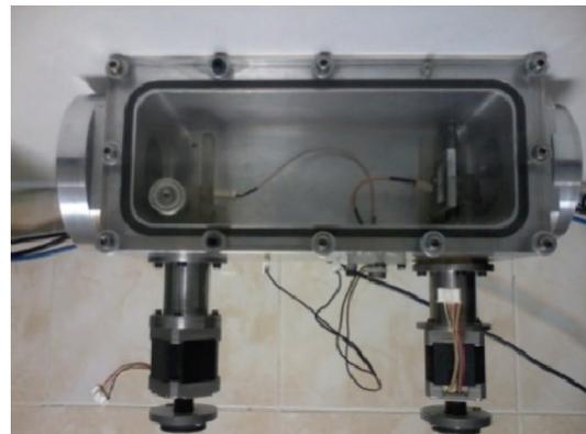
Fig. 11. (color online) A homemade emittance scanner composed of a cube with 15 cm length and width and a 35 cm height aluminum scanner box.
