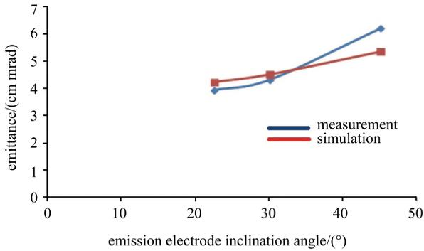
Fig. 12. (color online) Measured and simulated emittance as a function of emission electrode inclination angle.
