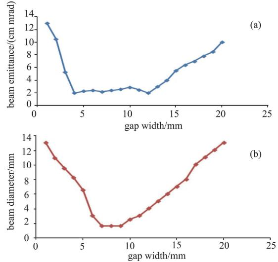
Fig. 7. Beam emittance (a) and beam diameter (b) as a function of the gap width of the emission and focusing electrode.
