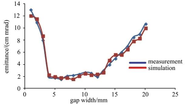
Fig. 14. (color online) Measured and simulated emittance as a function of gap width.
