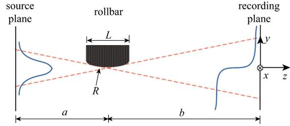
Fig. 2. Sketch of spot size measurement by the rollbar method.
