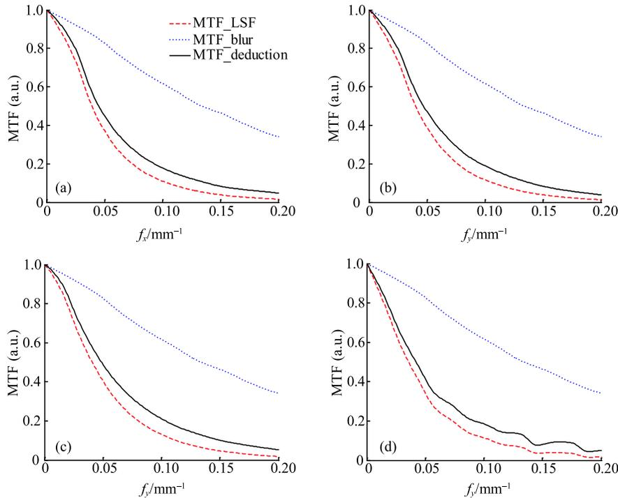
Fig. 6. MTF curves obtained in the spot size measurements by various techniques. (a) and (b) are the pinhole imaging method (No. 13031); (c) is the slit method (No. 13041); (d) is the rollbar method (No. 13044).
