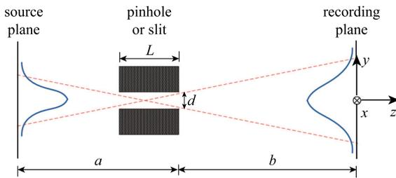
Fig. 1. Sketch of spot size measurement by the pinhole or the slit imaging method.
