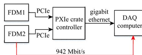
Fig. 6. Block diagram and result of data transmission test.
