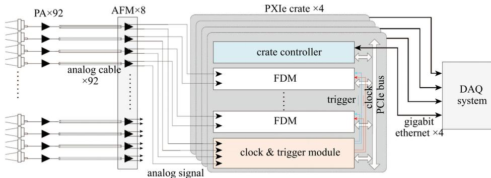
Fig. 1. Architecture of distributed readout electronics system.
