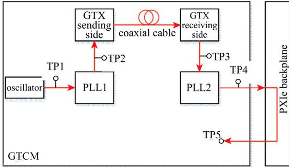
Fig. 7. Block diagram of clock performance test.
