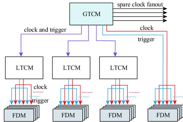
Fig. 4. Clock and trigger distribution network.
