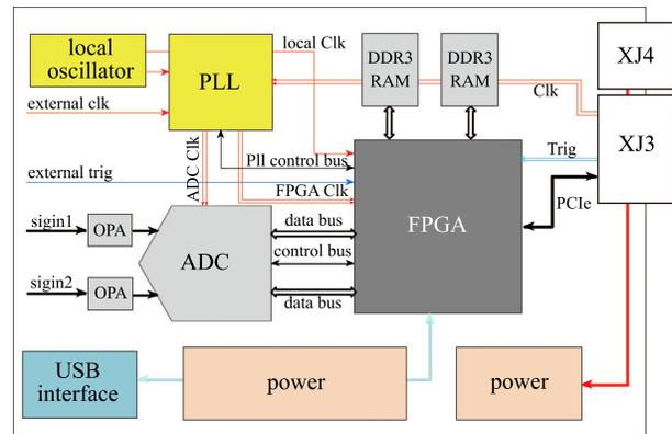
Fig. 2. Schematic of the field digitization module.
