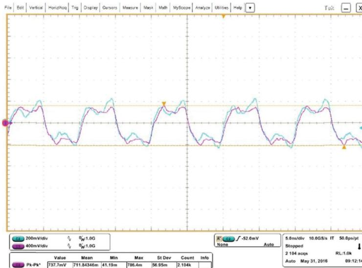
Fig. 8. Skew of the clock between different slots within a PXIe crate.
