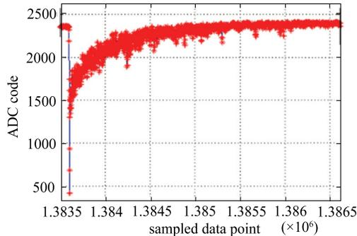
Fig. 10. Typical waveform for cosmic rays.
