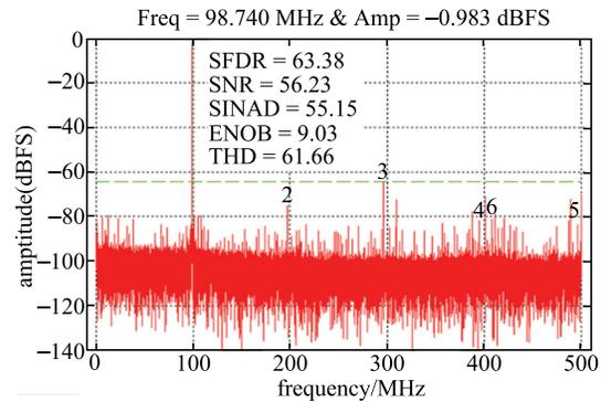
Fig. 5. Results of dynamic performance tests.
