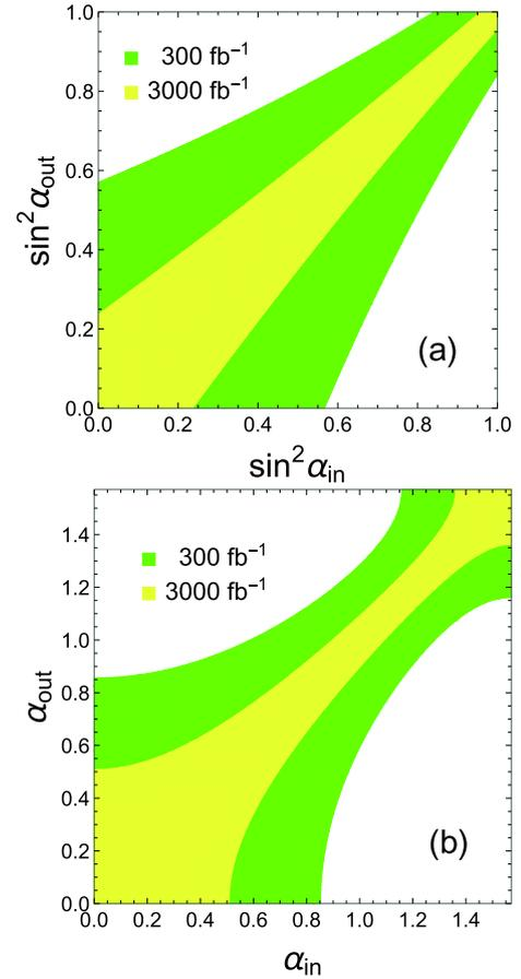
**Fig. 6.** (color online) Projected accuracy of the  $\alpha$  measurement versus the input value at the LHC with integrated luminosities of  $300 \text{ fb}^{-1}$  (green) and  $3000 \text{ fb}^{-1}$  (yellow), respectively.
