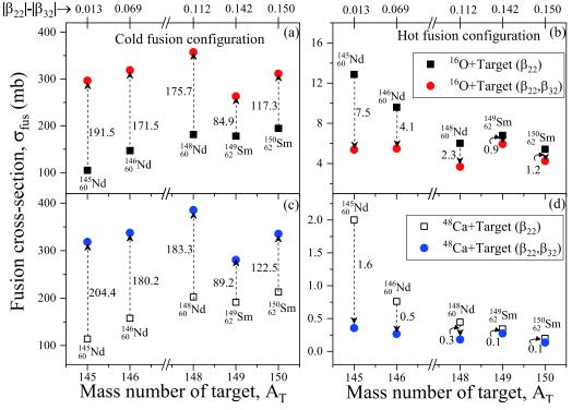
**Fig. 9.** (color online) The fusion cross-sections calculated using the Wong formula [39] for the (a), (c) cold and (b), (d) hot fusion configurations of the <sup>16</sup>O, <sup>48</sup>Ca+soft-pear shape (<sup>145,146,148</sup>Nd and <sup>149,150</sup>Sm) reactions, at  $E_{c.m.} = V_B$ .
