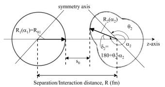
**Fig. 2.** Schematic configuration of spherical-plus-octupole axially symmetric deformed and oriented nuclei lying in the same plane.
