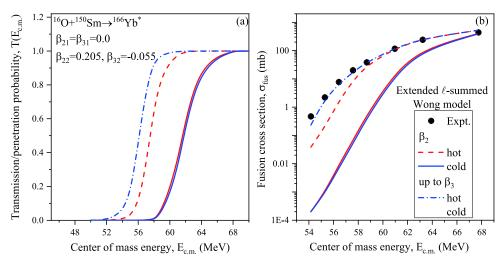
**Fig. 10.** (color online) (a) The transmission probability  $T(E_{c.m.})$  calculated as a function of the center of mass energy  $E_{c.m.}$  (MeV), and (b) fusion cross-sections obtained using the extended  $\ell$ -summed Wong model [47] for the  ${}^{16}O+{}^{150}Sm$  ( $\beta_{22} = 0.205, \beta_{32} = -0.055$ ) reaction [1] at both the hot and cold optimum orientations [36] related to quadrupole and octupole deformations across the Coulomb barrier energies.
