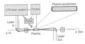
Fig. 4. Schematic layout of a laser-plasma acceleration laboratory.
