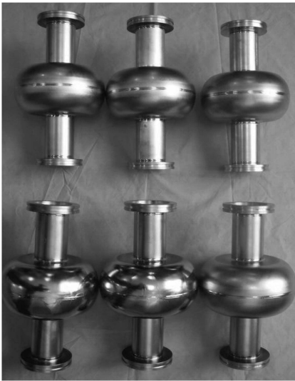
Fig. 1. Cavities with the IHEPLL shape fabricated at IHEP. (Top three: Tokyo Denki fine grain niobium. Bottom left two: China Ningxia LG Niobium; Bottom right: China Ningxia fine grain niobium).
