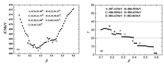
Fig. 1. Energy surface(a) and  $\gamma$  deformation as functions of deformation  $\beta$  in constrained triaxial calculation with PK1 for <sup>104</sup>Rh. The minima in the energy surface are presented and labeled by A-F with their corresponding deformation  $\beta$  and  $\gamma$  and energies.
