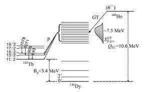
Fig. 2. Schematic representation of  $\beta$ -delayed proton decay of <sup>146</sup>Ho. The  $\gamma$  transitions are labeled with their energies in keV.
