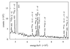
Fig. 1. The  $\gamma$  spectrum gated on the delayed protons with energies from 2.2 to 6.5 MeV.
