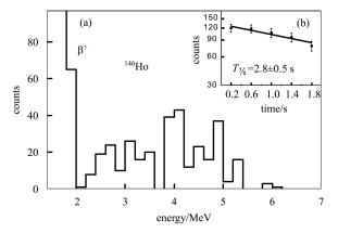
Fig. 3. (a) The energy spectrum of  $\beta$ -delayed protons gated on the 640 keV  $\gamma$  peak. (b) The time spectrum of the 640 keV transition gated by protons.
