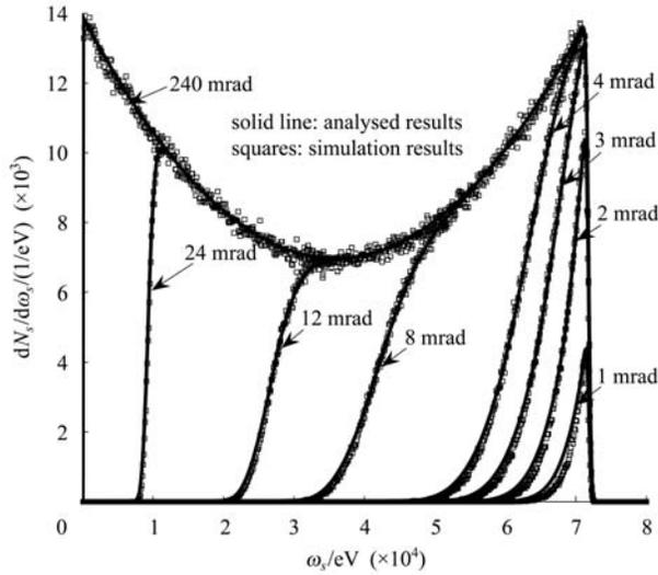
Fig. 3. Spectral distributions of the scattered photons for a Thomson scattering system obtained with different acceptance angles.
