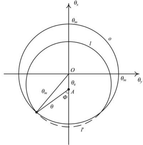
Fig. 1. Angular geometry of Thomson scattering. Circle  $O$  represents the acceptance range of the detector, and dot  $A$  represents an electron with an incident angle  $\theta_e$ . Arc  $l$  represents the scattered photons with direction angle  $\theta$  that are received by the detector, and arc  $l'$  represents those out of the acceptance range.
