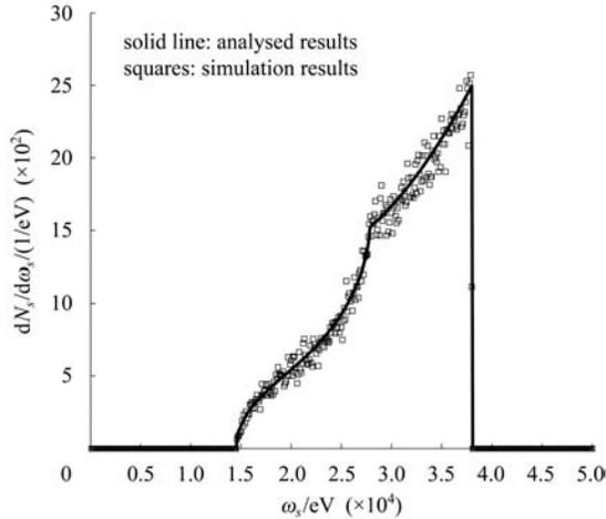
Fig. 2. Spectral distributions of the scattered photons obtained with acceptance angle  $\theta_m = 4.2$  mrad. Here the electron energy is 40 MeV, the laser wave length is 800 nm, the laser energy is 1 J, the laser radius is 20  $\mu\text{m}$ , the laser length is 1ps, and the incident angle of the electron and the laser beam  $\theta_e = 3$  mrad.
