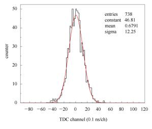
Fig. 5. The time resolution of the LPMWPC.
