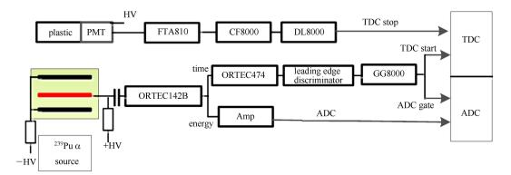
Fig. 3. The time resolution measurement system.
