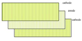
Fig. 1. Structure of the LPMWPC.
