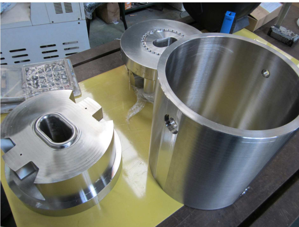
Fig. 2. The three unassembled parts of the LFB kicker.
