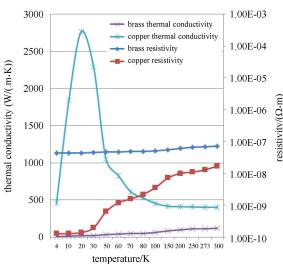
Fig. 4. Electric resistivity and thermal conductivity of pure copper and brass.
