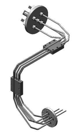
Fig. 5. 3D engineering drawing of the current lead.
