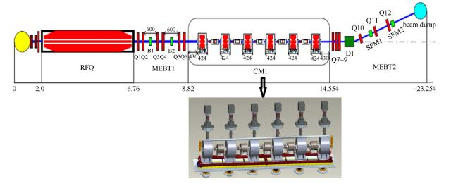
Fig. 1. Schematic layout for ADS injection I and the detailed cryomodule.
