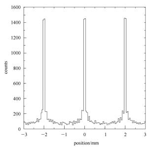
Fig. 4. Calculated uniform irradiation response of a detector with cathode wire spacing of 1 mm.
