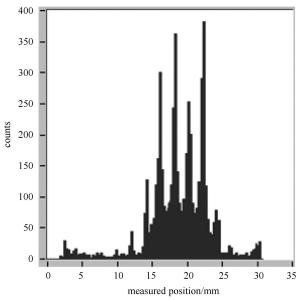
Fig. 5. Measured position response of the detector for a collimated X-ray beam.
