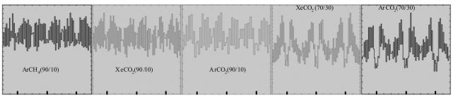
Fig. 8. Best UIR spectrum of the detector using different working gases with drift region depth of 12 mm; the markers on the *x*-axis represent the positions of the anode wires.
