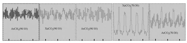
Fig. 7. Best UIR spectrum of the detector using different working gases with drift region depth of 20 mm; the markers on the *x*-axis represent the positions of the anode wires.
