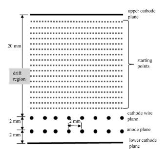
Fig. 1. Structure of the MWPC.
