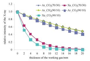
Fig. 3. (color online) X-ray attenuation in different gas mixtures.
