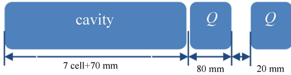
Fig. 3. (color online) Layout of the focusing structure.
