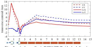
Fig. 5. (color online) IMPACT-T (dashed lines) and ASTRA (solid lines) beam trajectory comparison with an identical magnetic field strength.
