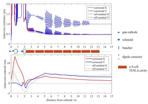
Fig. 6. (color online) Results of the joint-ASTRA-IMPACTT simulation program including 3D SC calculation, for emittance (top figure) and centroid (bottom figure) evolution of optimized corrected beam, and the uncorrected beam.
