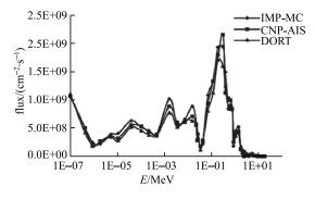
Fig. 13. Neutron flux spectrum at capsule location.
