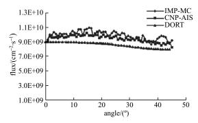
Fig. 11. Neutron cavity flux (E > 0.1 MeV).
