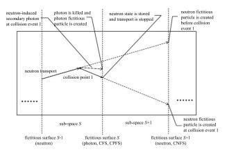
Fig. 3. Particle transport in the CNP-AIS method.
