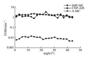
Fig. 16. FOM curves of neutron flux at pressure vessel 1/4 peak axial location (E > 1.0 MeV).
