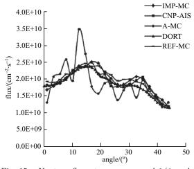
Fig. 15. Neutron flux at pressure vessel 1/4 peak axial location (E > 1.0 MeV).
