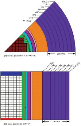
Fig. 4. (color online) PWR model with full size biological shield wall (all dimensions in cm; the other parts of this model refer to Ref. [12].
