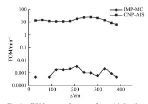
Fig. 9. FOM curves of neutron flux axial distribution in biological shield wall.
