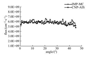
Fig. 12. Photon cavity flux (E > 0.1 MeV).
