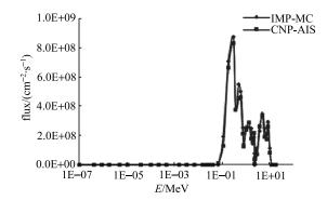
Fig. 14. Photon flux spectrum at capsule location.
