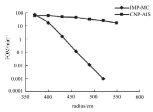
Fig. 5. FOM curves of neutron flux radial distribution in biological shield wall.
