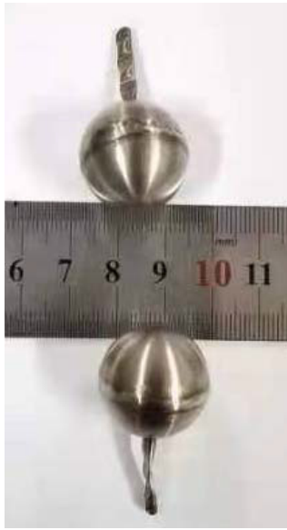
Fig. 2. (color online) Photograph of the high-pressure spheres used in this work.
