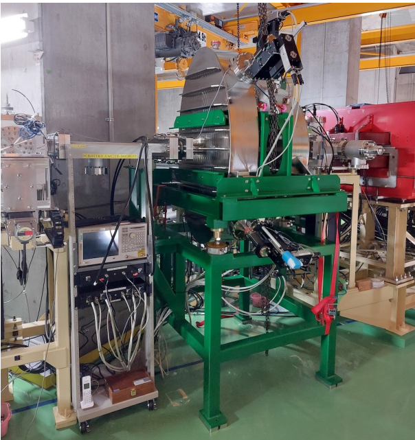
Fig. 1. (color online) Photograph of a Schottky Cavity Doublet (SCD) installed at the R3 storage ring. It is on top of a green mechanical support (elliptical cavity left). A separate publication will be dedicated to the technical details and features of the new detector (Photo: S. Sanjari).
